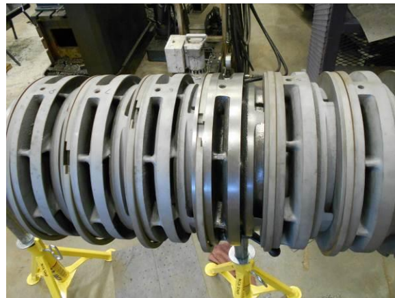
Figure 12: Diffusers on Shaft
