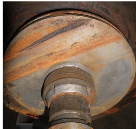
Figure 2: Original Impeller Condition on Shaft
