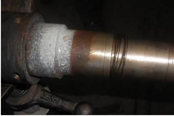
Figure 13: Paint on Shaft to be Removed
