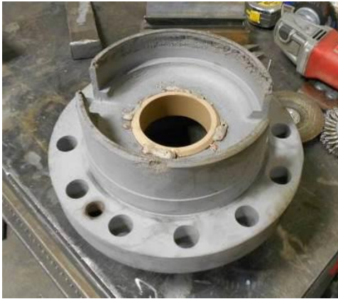
Figure 34: Stuffing Box Extension with Erosion
