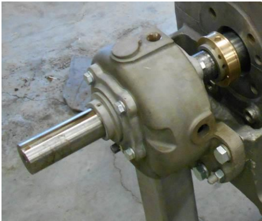
Figure 15: Drive End Shaft Repaired
