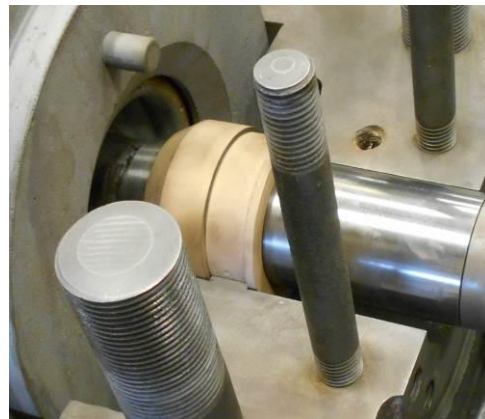
Figure 37: Drive End Bushing on Shaft
