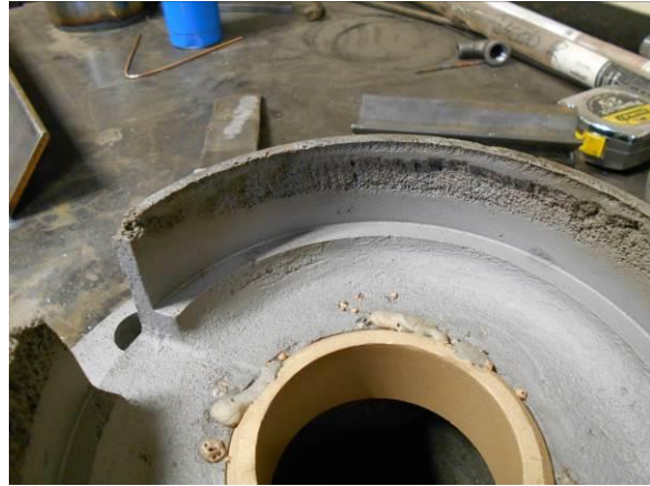
Figure 35: Close Up of Erosion
