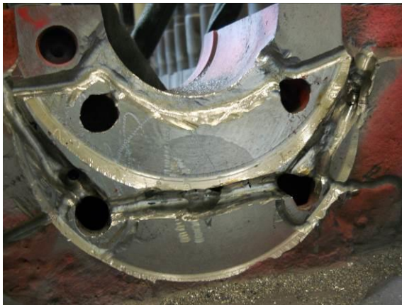
Figure 25: Water Jacket Excavated and Cleaned Out
