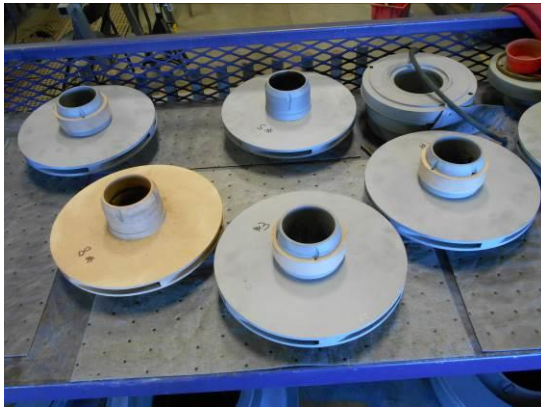
Figure 5: Impellers Sand Blasted
