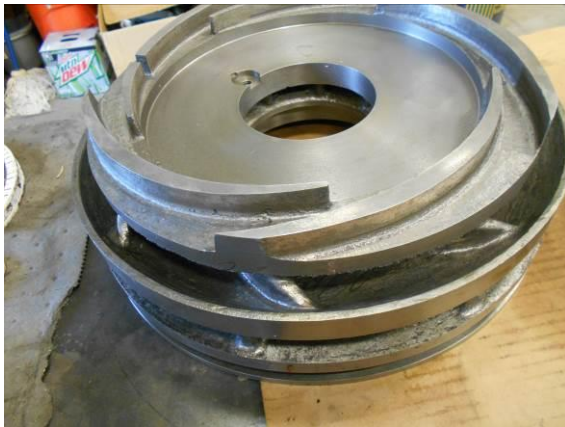
Figure 11: New Diffuser Stacked on Sand Blasted Diffusers
