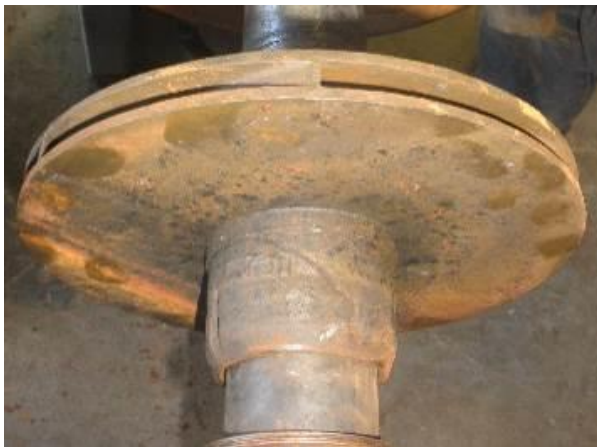
Figure 1: Original Impeller Condition on Pump Shaft
