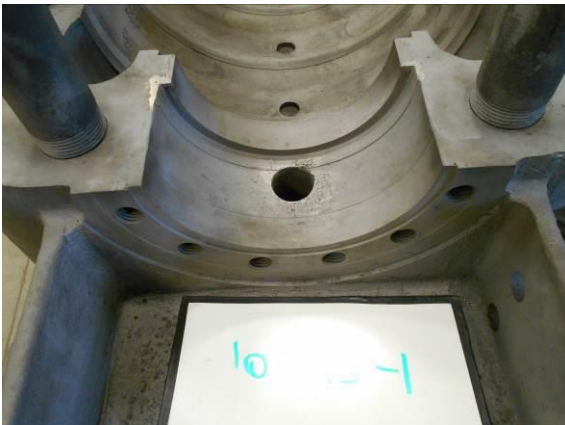
Figure 29: Thrust End Bottom Corners Repaired
