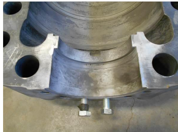
Figure 30: Thrust End Top Corners Repaired
