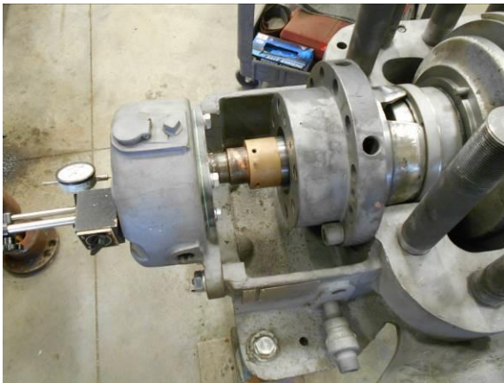
Figure 36: Stuffing Box Extension on Shaft
