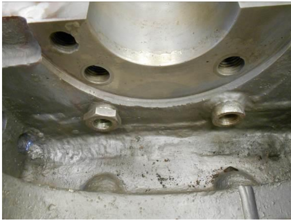
Figure 27: Water Jacket Repaired and Machined
