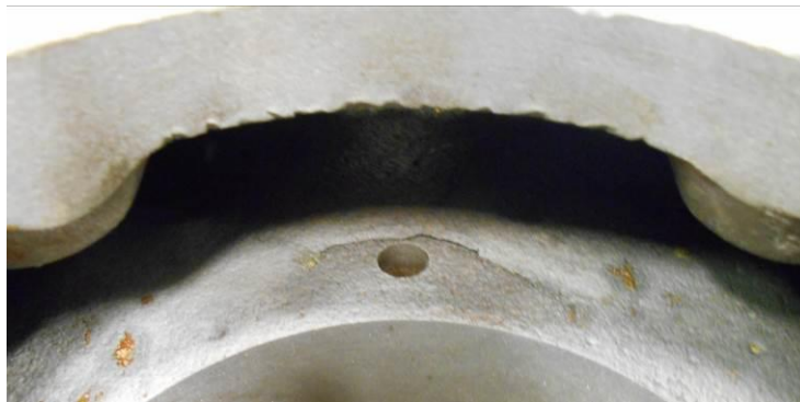
Figure 42: Crack in Bearing Housing
